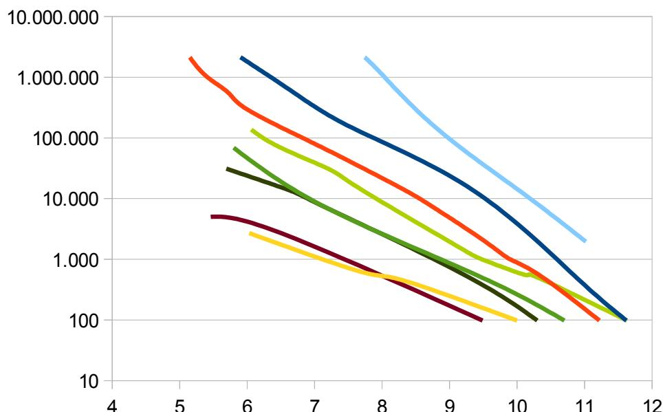
GPC-calibration curves AppliChrom ABOA StyDiViBe 300x8mm, THF, 1ml/min, PMMA standards, M[Da] vs.  $V_e$  [ml], porosities: 35A, 100A, 500A,  $10^3$ A, 1500A-BPT,  $10^5$ A-BPT,  $10^6$ A-BPT,  $10^7$ A-BPT
