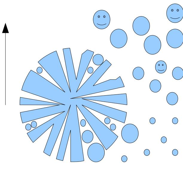
Conventional GPC technology: combining columns of various pore sizes or by combining different pore sizes in one column enlarges the calibration range – but it can lead to artifacts in the exact calibration of the GPC system that reduces molecular size accuracy determination
