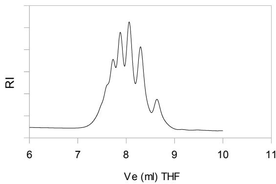
GPC calibration curve AppliChrom ABOA StyDiViBe 35A BPT 300x8mm (large pore volume plus low exclusion limit for high oligomer resolution even with low backpressure); safe money plus increase resolution
