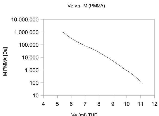
AppliChrom ABOA StDiViBe 10E5A BPT-Technology: Large calibration range respective good to calculate calibration curve from monomer up to 1.5Mio Dalton, ideal technological step ahead if a combination of porosities results in „artificial shoulders“ of calibration curves and/or in artificial shoulders of broad distributed molecular weight polymers. An easy to use tool to improve quality of results for your analytes.
