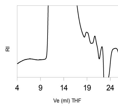
AppliChrom BPT Technology: a combination of small, medium and large pores in each particle ensures an increase of calibration range. No matching porosities effects – respective artificial shoulders in chromatogrammes known from many column combinations are significantly reduced – for improving your GPC Chromatography.
