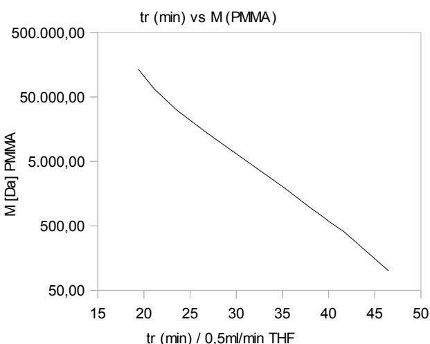
Good resolution, calibration range respective linearity in the range of 100-120.000Da, obtained from the special AppliChrom BPT-technology. No „surprising“ porosity artefacts from mixing particles with pores of different size for covering the full range of molecular sizes. Great resolution even if 8µl RI measuring cell is used.
